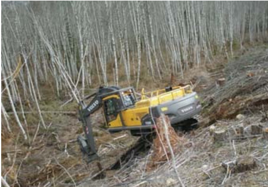
The LevelMax function needs more than its full 21° to cope with this decline
