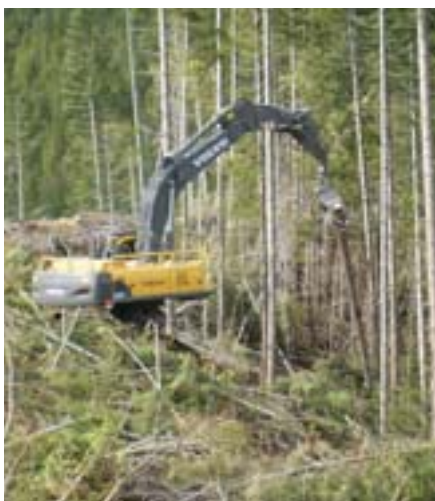
This TFC levels out on a steep slope using the LevelMax module
