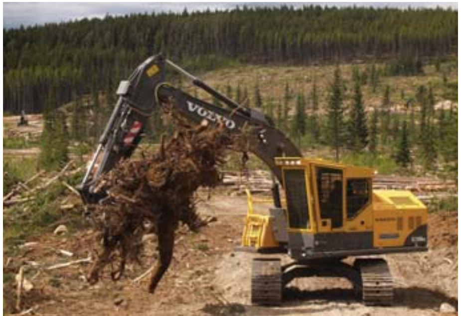
The FC2421C splits stumps in Finland
