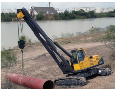
Excellent stability and traction enable working on up to 35° grade slopes.
