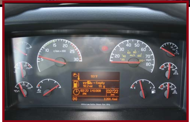
The Volvo dash has two liquid gauges flanking the driver display. On the right side is fuel; the left side is for the diesel exhaust fluid, or DEF.
